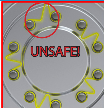
Danger - wheel nuts have loosened!
